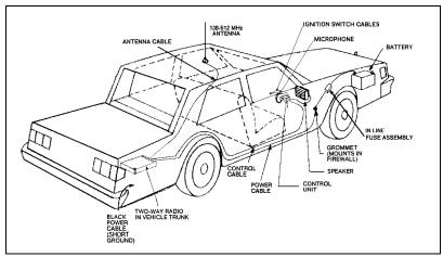
**Figure 4 - Typical Installation (Remote Mount Shown)**
